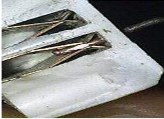
Fig:5.14 Inside of a solderless breadboard strip
