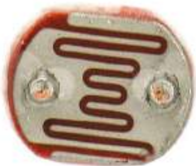
Fig:5.34 19M51 LDR top view.
