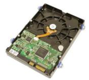
The hard drive is where your software, documents, and other files are stored. The hard drive is long-term storage, which means the data is still saved even if you turn the computer off or unplug it.
