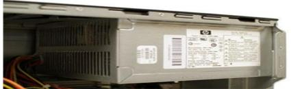
The power supply unit in a computer **converts the power** from the wall outlet to the type of power needed by the computer. It sends power through cables to the motherboard and other components.
