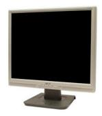
The **monitor** works with a **video card**, located inside the computer case, to display images and text on the screen. Most monitors have **control buttons** that allow you to change your monitor's display settings, and some monitors also have built-in speakers.
