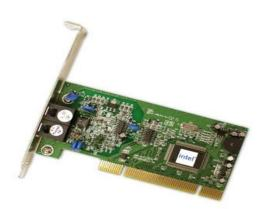
The **network card** allows your computer to communicate over a network and access the Internet. It can either connect with an **Ethernet** cable or through a **wireless** connection (often called **Wi-Fi**). Many motherboards have built-in network connections, and a network card can also be added to an expansion slot.
